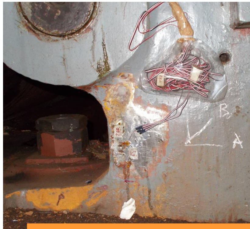
Foundation Bolt Reactions
